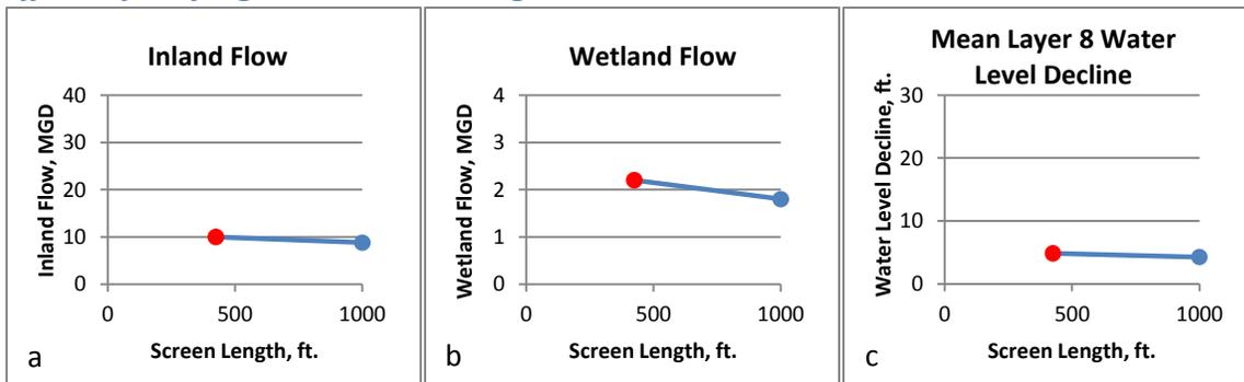
Figure 4. Effects of slant well screen length on inland flow (a), wetland flow (b), and mean Layer 8 water level decline (c).
