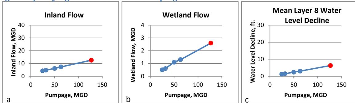
**Figure 6. Effects of changes to the slant well pumping rates on inland flow (a), wetland flow (b), and mean Layer 8 water level decline (c).**
