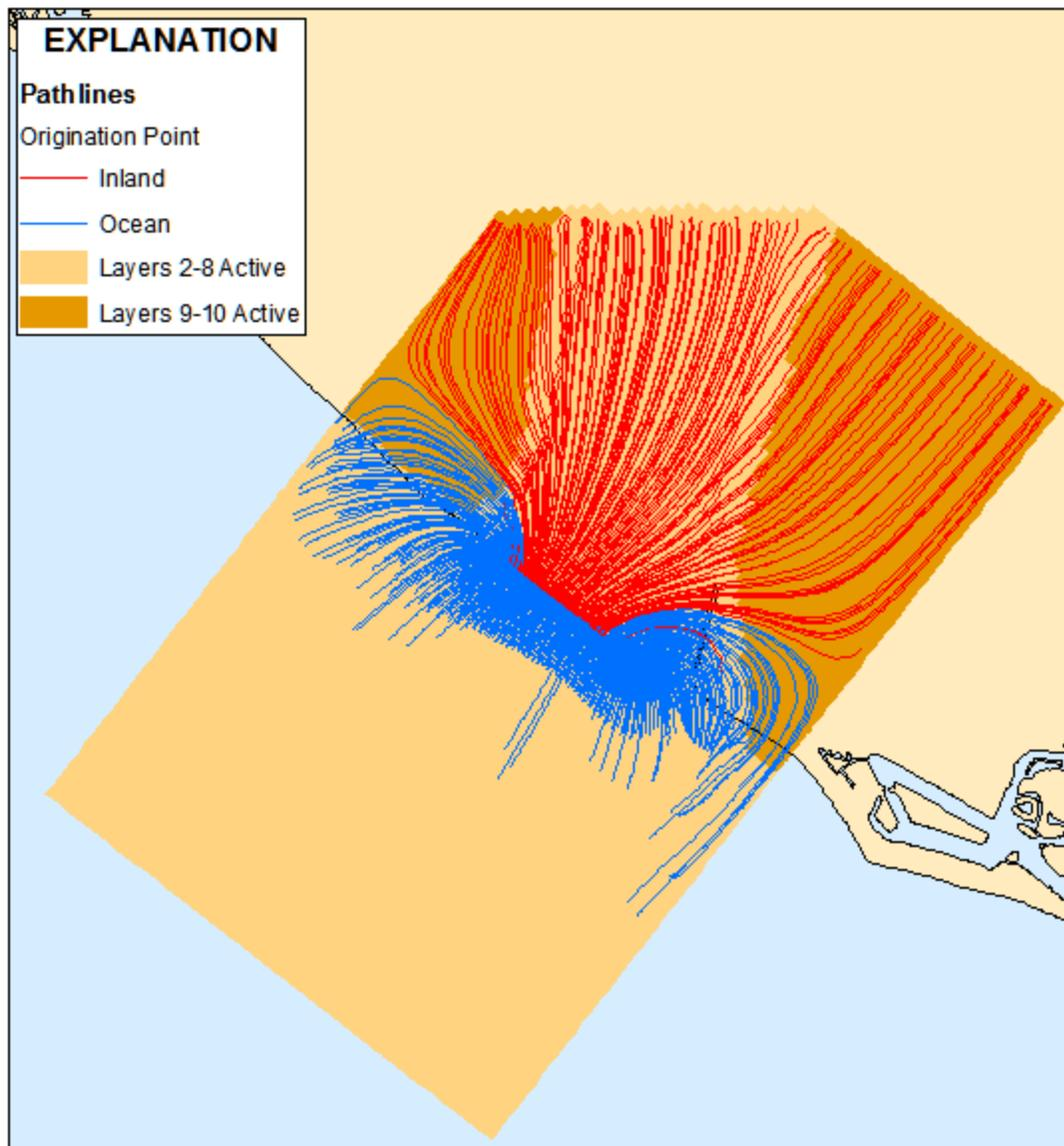
Figure 8. Groundwater flow paths to the slant wells.
